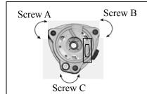
Turn the instrument approximately 90°. Adjust screw C, till the bubble in the center of the level.
