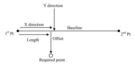
Length: Distance along the baseline from 1<sup>st</sup> point to the position at which a line extending from the required point intersects the baseline at right angles (X direction) Offset: Distance from the required point to the position at which a line extending from the required point intersects the baseline at right angles (Y direction).
