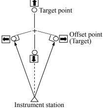
When the offset point is positioned to the left or right of the target point, make sure the angle formed by lines connecting the offset point to the target point and to the instrument station is almost 90°.
