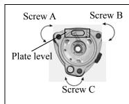
Loosen the horizontal motion clamp, and turn the instrument till the plate level is parallel to a line shaped with screws A and B. Adjust the screws A and B to make the bubble in the center of the level.
