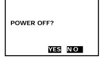
Press  $\{\text{POWER}\}\$  key, the instrument will ask you to turn off the instrument or not, press F3(Yes), it will be turned off, press F4(No) back to previous screen.
