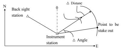
[Procedure of coordinate stake out measurement]
